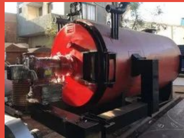
Thermal Fluid Heater for Chemical Industry
