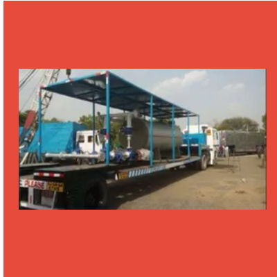
Oil & Gas Fired 1000 kg/hr Mobile Boiler System (MBS)
